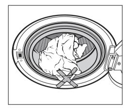
To prevent damage to the door seal and clothing, make sure that there are no clothes caught between the drum door and the seal.
